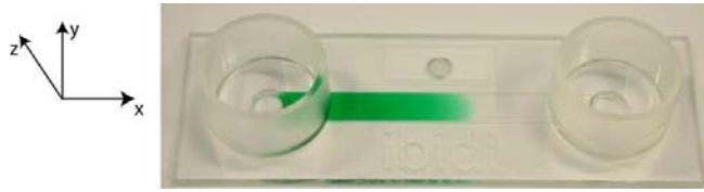
Fig. 2: Image of gradient visualized by food coloring. Make sure the colored solutions are identical in density. If not, the colored and non-colored liquid may flow into each other in a non-defined way.
