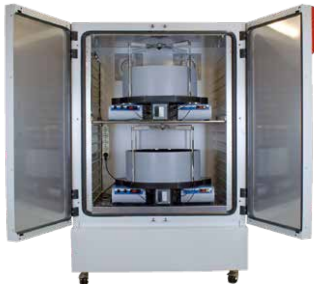
Thermal Conditioned Cabinet for Thermal Gradient Ring
