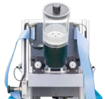
Pellet dispenser (for each chamber)
